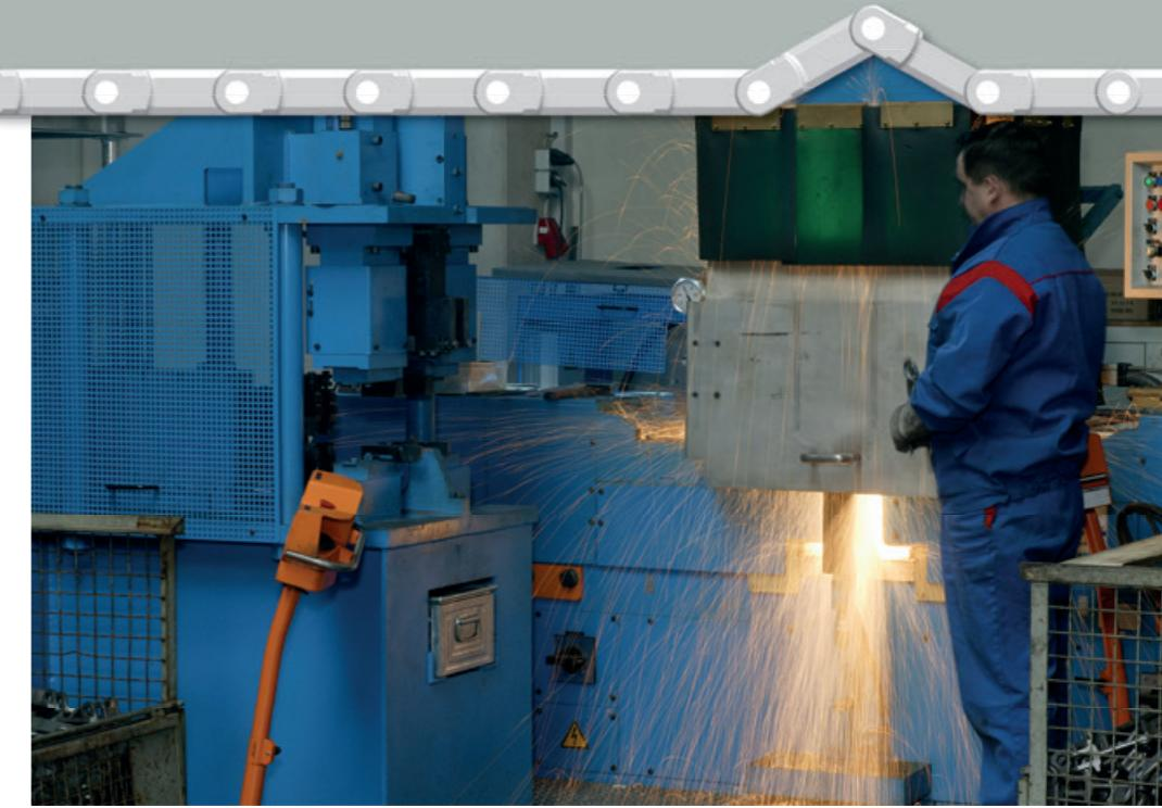
To optimize the welded connection between chain link and flight we use a customized flash-butt welding machine with integrated deburring device according to DIN 44752. Flash-butt welding is a computer-aided welding procedure with parameter-logging. As impairment of the chain links, caused by irregular preheating that could lead to crack formation is precluded this is the technical optimal solution.
